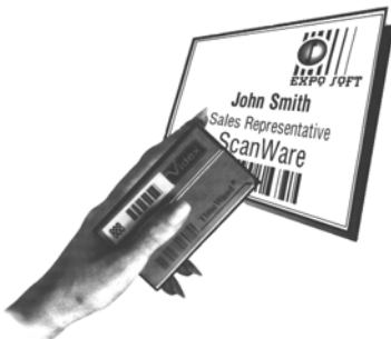
HOLD THE EZ❖TRAC™ SCANNER COMFORTABLY IN YOUR HAND, MAKING SURE THE CORNER WITH THE OPTICAL SENSOR IS POINTING AT THE BAR CODE
